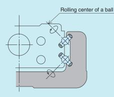
Fig.4 Contact Structure of SKR-Type
