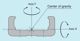
Fig.3 Sectional View of Outer Rail
