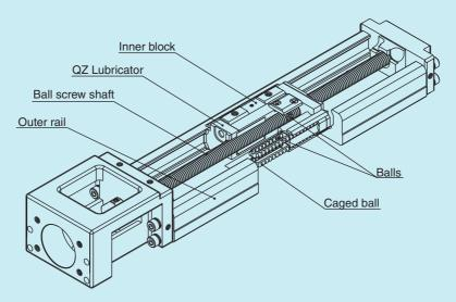
Fig.1 Construction of SKR-type LM Guide Actuator with Caged Ball Technology
