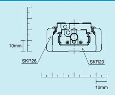
Fig.5 Cross Section of SKR-Type
