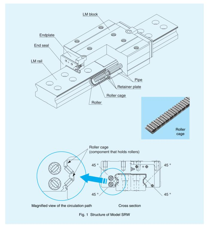
Based on Roller Guide with Caged Technology model SRG, this model has a wider rail and two rows of LM rail mounting holes to achieve high mounting strength and mounting stability. Use of the roller cage allows low friction and smooth motion. Thus, model SRW is an ultra-high rigidity Roller Guide that achieves long-term maintenance-free operation.
