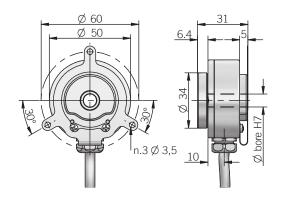
recommended mating shaft tolerance g6 dimensions in mm
