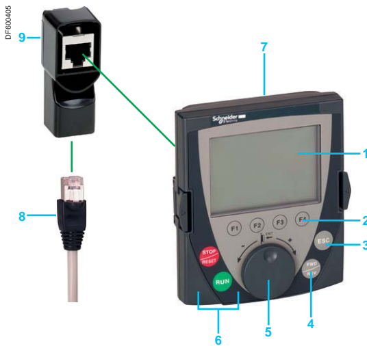
Graphic display terminal + remote-mounting cordset + female/female RJ45 adaptor
