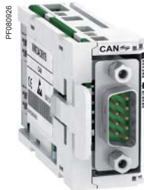
VW3 A3 618 CANopen communication card
