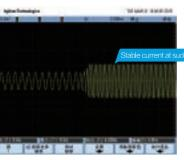
Current waveforms when sudden loading in vector control mode with 0.5Hz and full load
