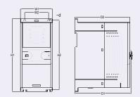
Wall mounting of 0.75~2.2kW VFDs
