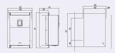
Flange mounting of 3PH 380V 90~110kW VFDs
