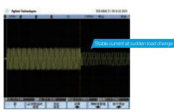
Current waveforms when sudden unloading in V/F control mode with 2Hz and full load
